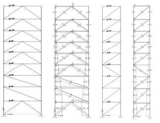
DESIGN OF CHEVRON AND DIAGONAL BRACED FRAMES METHODOLOGY
